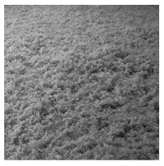
ThermaGlas® Fiber Glass Loosefill Insulation is an alternative to roll or batt insulation in attics, new construction and retrofit applications.
